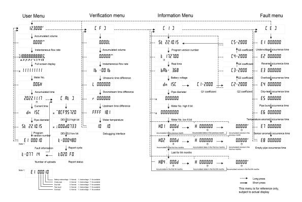
Note: The LCD display can be customized according to customer's requirement.
