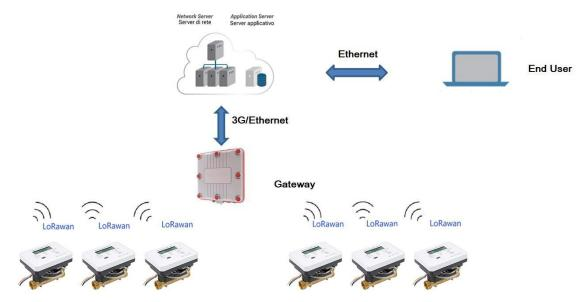
The whole system mainly consists of LoRaWAN Wireless Network + LoRaWAN Gateway
